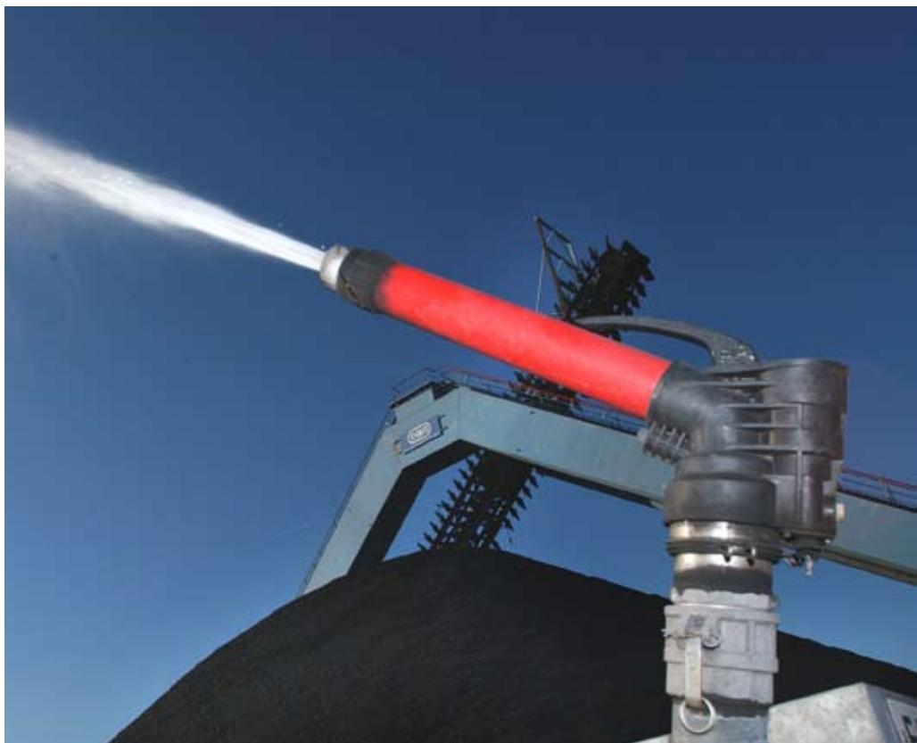
Dust is produced wherever bulk material like sand, coke, coal, mineral ore is handled or stored. This dust is a burden for nature and humans in equal measure. Dust suppression on bulk material processing plants has become an absolute must to protect environment, nature and humans.
